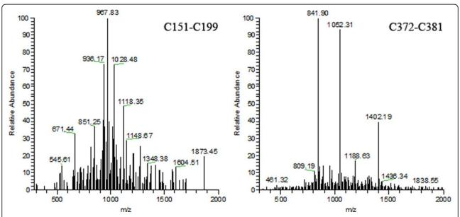
**Figure 1 Tandem mass spectra for protein C2GnT-I**. (Left) Confirmatory spectrum for disulfide bond C151-C199 for protein C2GnT-I (chymotryptic digested). (Right) Confirmatory spectrum for disulfide bond C372-C381 determined for protein C2GnT-I (tryptic digested).
