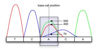
**Chromatogram trace showing peak intensities where dashed line is the base-call position**. Three peaks are detected at this position. The intensities of green, red, and blue peaks are 500, 400, and 70 units, respectively and are used in peak intensity ratio calculation.
