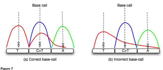
**Effect of signal intensity decay on base-calling**. Correct (a) and Incorrect (b) base-calling interpretation due to signal intensity decay.
